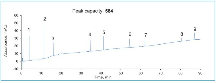
With a HALO® 2.0  $\mu$ m 160 Å ES-C18 column, very high peak capacity values can be obtained within 90 minutes. The sharp, narrow peaks facilitate separations of complex, challenging samples, such as tryptic digests.
