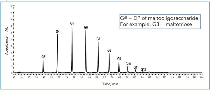
A HALO® Glycan column shows an efficient separation of procainamide-labeled dextran standards (Sigma-Aldrich 1:1 (w/w) of part numbers 00268 and 00269) at 0.5  $\mu$ g/ $\mu$ L in 70% ACN/30% water. Each lot of HALO® Glycan packing is tested using this sample to assure lot-to-lot reproducibility and performance.
