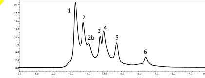
Column: HALO 1000Å C4, 2.1 x 150 mm: Flow rate: 0.1, 0.2, 0.4, or 0.6 mL/min: Mobile Phase A: 88/10/2 water/AcN/n-propanol/0.1% TFA
