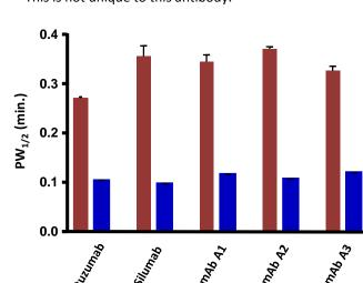
• For all mAbs tested, the peak widths measured at 50% peak width were smaller with the 1000Å SPPs compared to the 300Å FPPs
