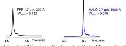
Improved resolution of an IgG1 (trastuzumab) is demonstrated by the 2.7 μm particle with 1000 Å pores. This is not unique to this antibody.
