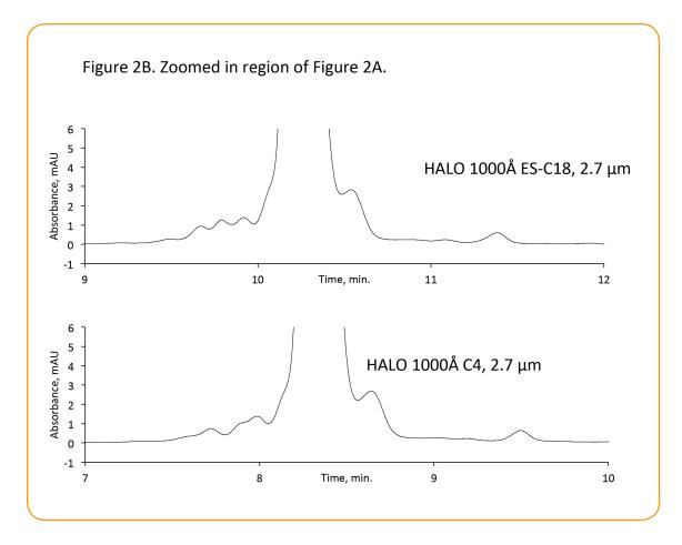
In Figure 2B, increased resolution of the minor components eluting before the major component of the NISTmAb is observed with the HALO 1000Å ES-C18 column compared to the HALO 1000Å C4 column. Identification and quantification of these minor components are often part of the quality control protocol used for the manufacturing of biotherapeutics.
