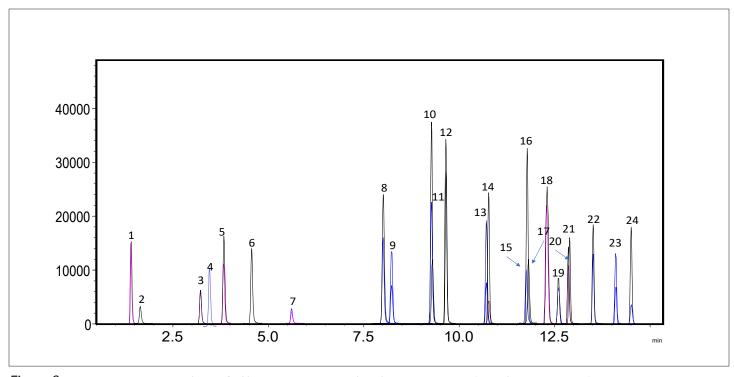
Figure 3. 24 target PFAS compounds specified by EPA 8327 separated on the HALO® PFAS Delay and HALO® PFAS columns.
