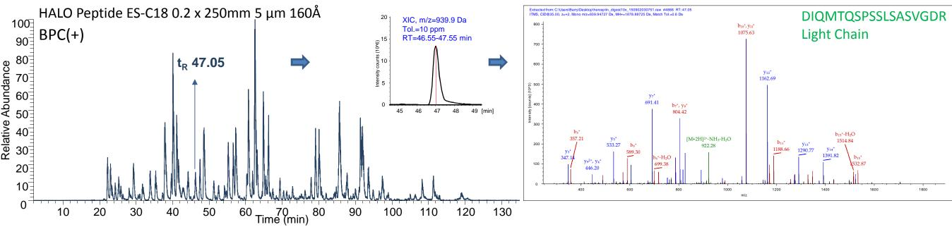
Two 250x0.2mm columns in series. Thermo Orbitrap Velos Pro/Dionex Ultimate 3000 UHPLC. 5µL injection of 3 µg/µL Trastuzumab tryptic digest. A = 0.1% DFA, B = 0.1% DFA in ACN. Loading Pump:  $2\%B @ 10\mu L/min$ . EXP stem cartridge  $33\mu I$  HALO C4. NC Pump: 5-55%B in 182min @  $3\mu L/min$ ,  $60^{\circ}C$ , • LC/HRAM MS is permitting evaluation of structures that are resolved, but it is
