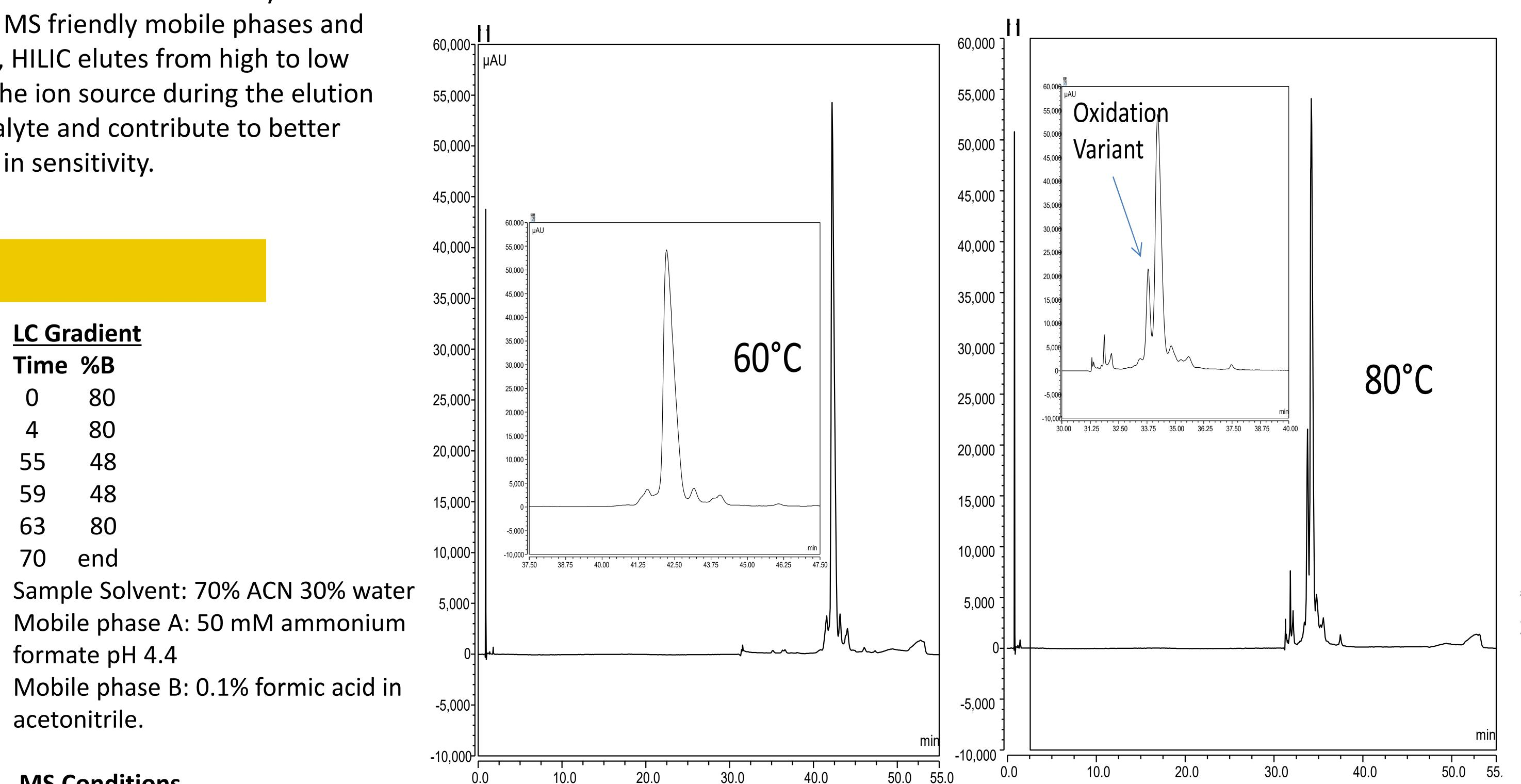
Figure 2. A) UV spectra of NIST mAb run at 60° C. B) UV spectra of NIST mAb run at 80° C showing oxidation artifact
