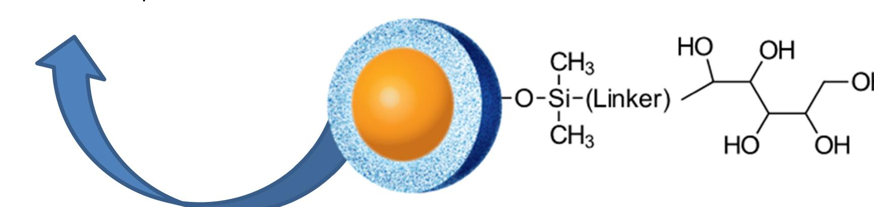
Figure 1. HALO® SPP particle and Penta-HILIC ligand structure
