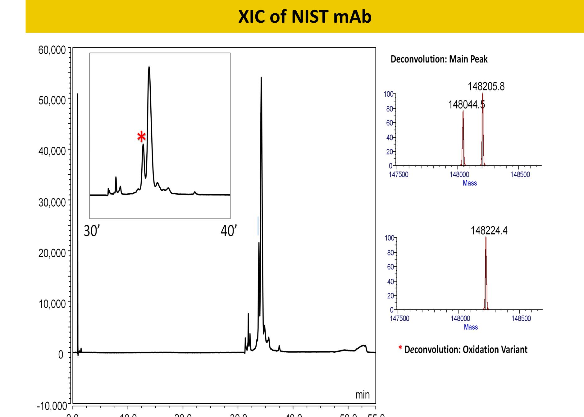
Figure 3. XIC of NIST mAb run at 80° C showing oxidation artifact and deconvoluted spectra
