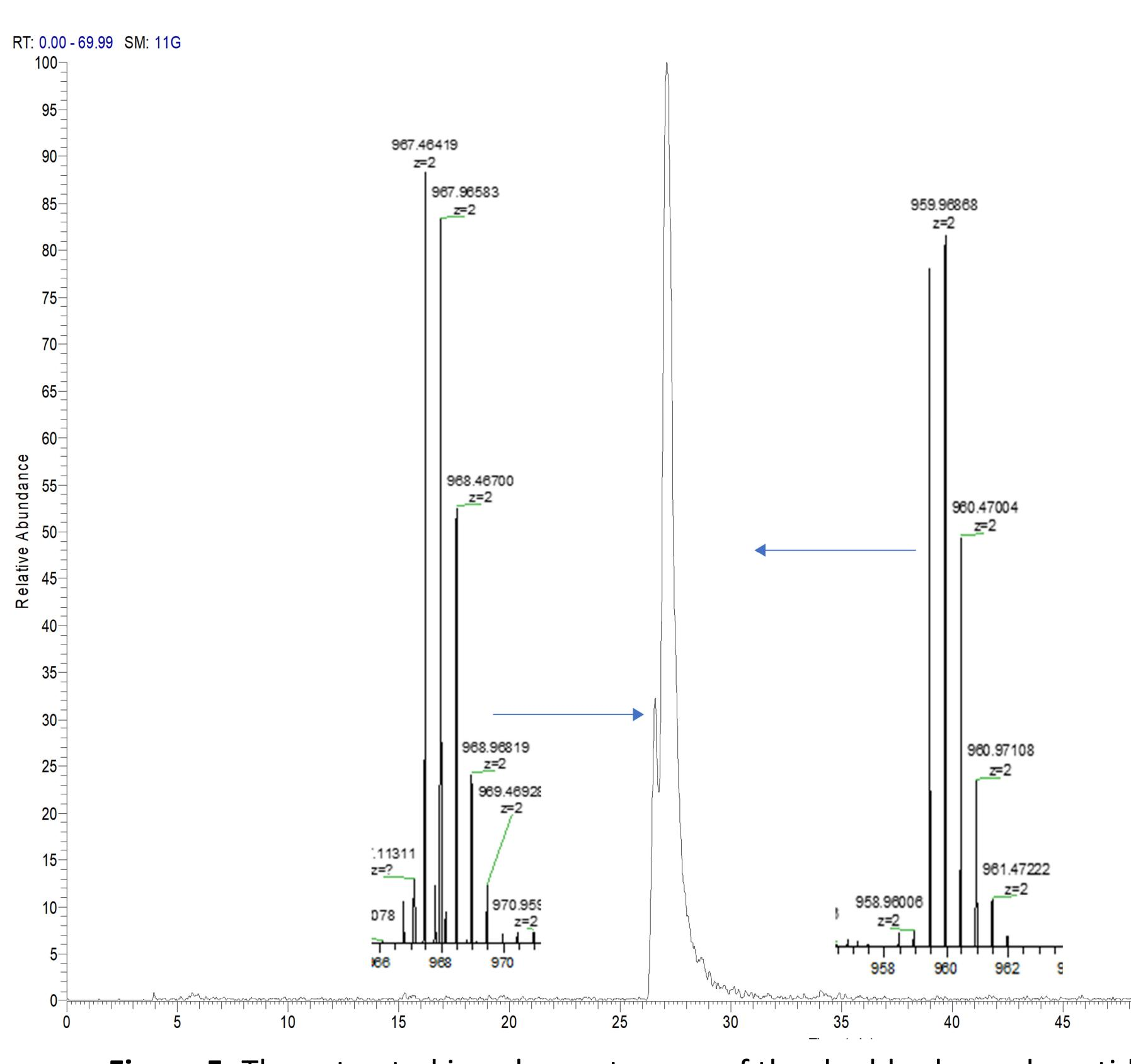
Figure 5. The extracted ion chromatogram of the doubly charged peptide fragment (R)EPQVYTLPPSREEMTK(N) showing a mass shift of 8.
