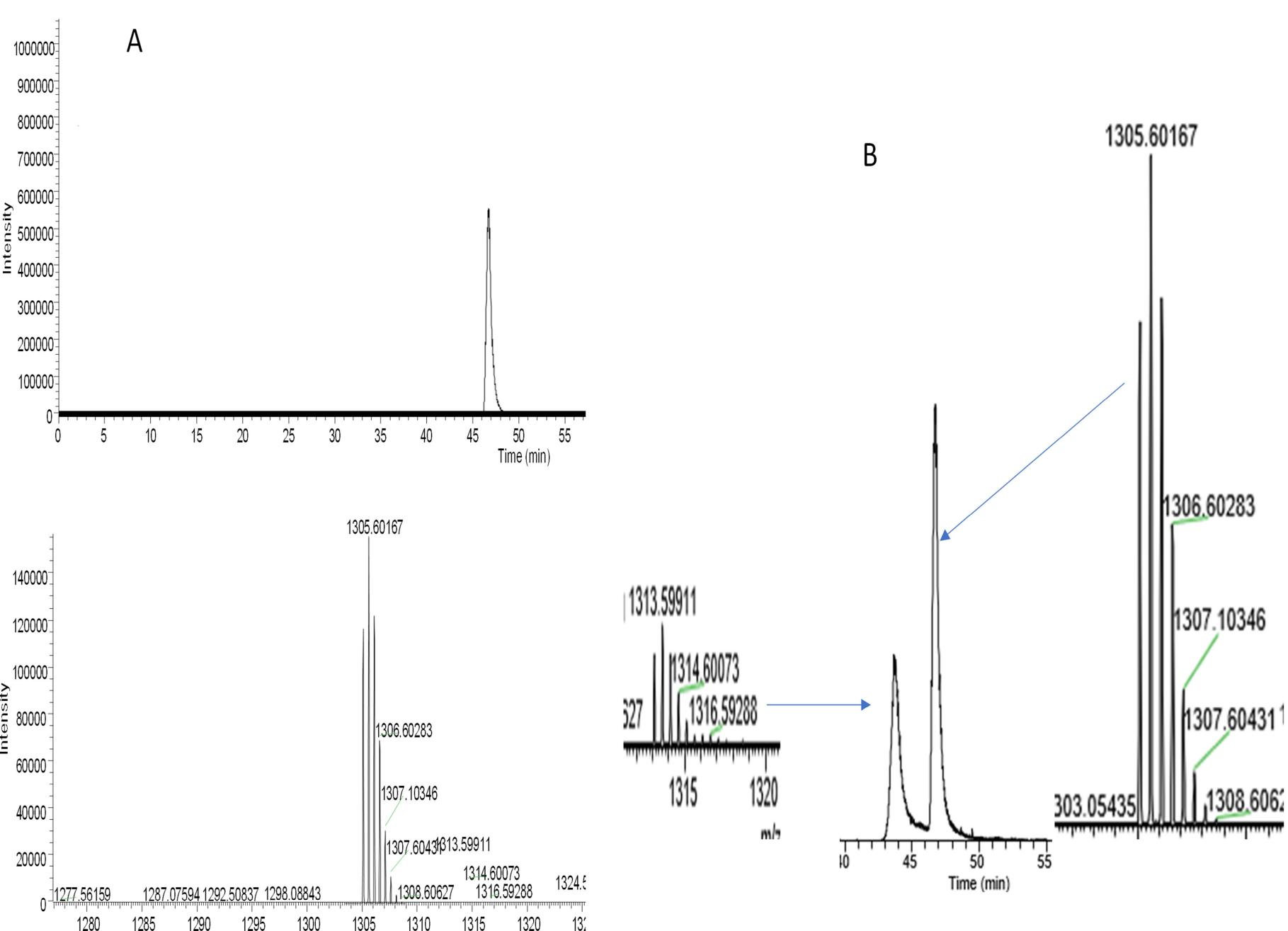
Figure 4. A) XIC of (-) DIQMTQSPSSLSASVGDRVTITC(Carbamidomethyl)R(A), m/z=1305.60167, before the oxidation experiment. B) XIC after the oxidation and shows the characteristic mass shift of 8 Da associated with oxidation for a doubly charged peptide species.
