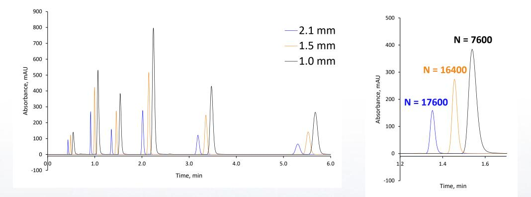
In move from 2.1 mm I.D. to 1.0 mm I.D., signal increases, but there is a significant loss in efficiency primarily due to extracolumn effects.
