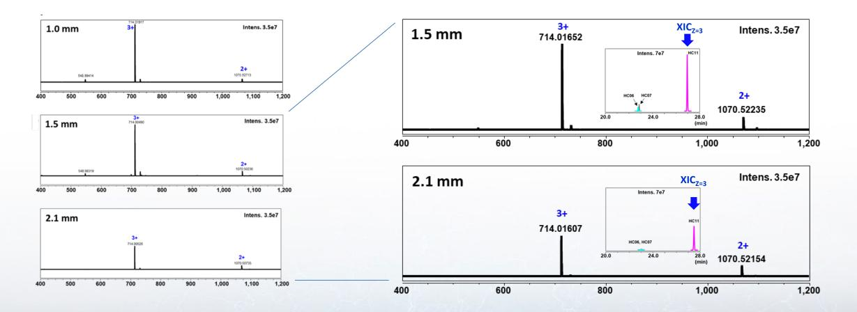
0.3µg trastuzumab tryptic digest, 2-50%B in 60 min 60°C ES-C18 150mm 2.7µm 160A; (A) 0.1%DFA H2O (B) 0.1%DFA ACN (*Gradient Delay*) Adapted from Fig. 4 B.P. Libert, J.M. Godinho, S.W. Foster, J.P. Grinias, B.E. Boyes, Implementing 1.5 mm internal diameter columns into analytical workflows, J. Chromatogr. A, 1676 (2022) 463207
