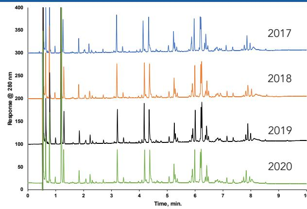
All new HALO® products are subject to stability testing. In this example the test required at least 1,000 injections at high temperature to demonstrate repeatability and performance. As shown, at 3,000 injections (approximately 23,000 column volumes) the results illustrated no significant changes in peak shape or retention.
