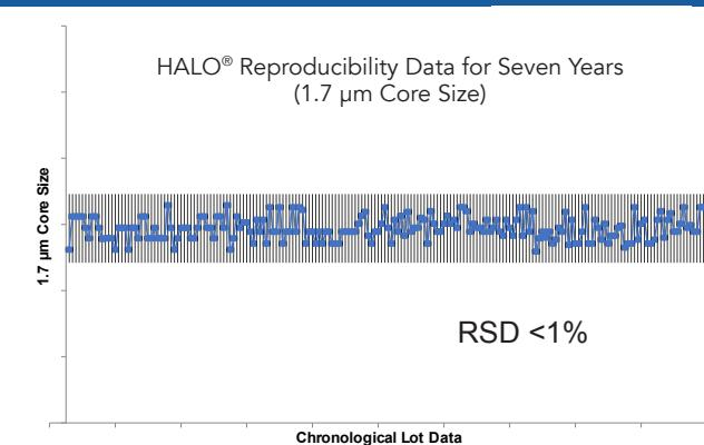
AMT's tight control of particle size distribution to RSD's of <1% highlights the quality control in our manufacturing processes. This narrow distribution ensures delivery of highly efficient columns.
